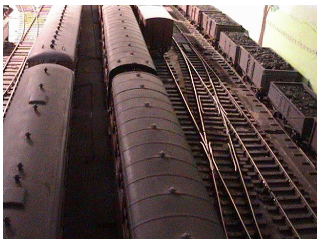
The facing crossover.
